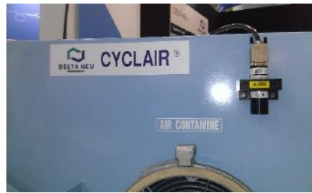
Filter radiological control system (certified EDF)
